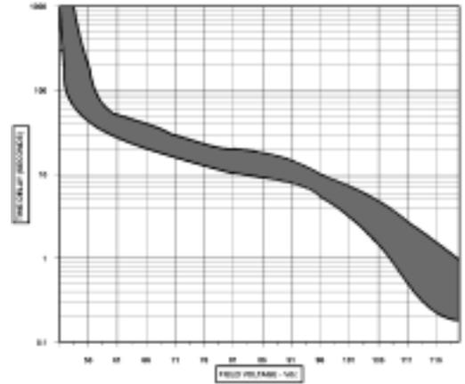
Figure 2. Typical Inverse Time Delay Characteristic Curve
