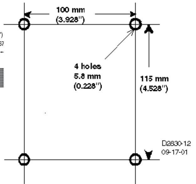
Figure 4. Drilling Template
