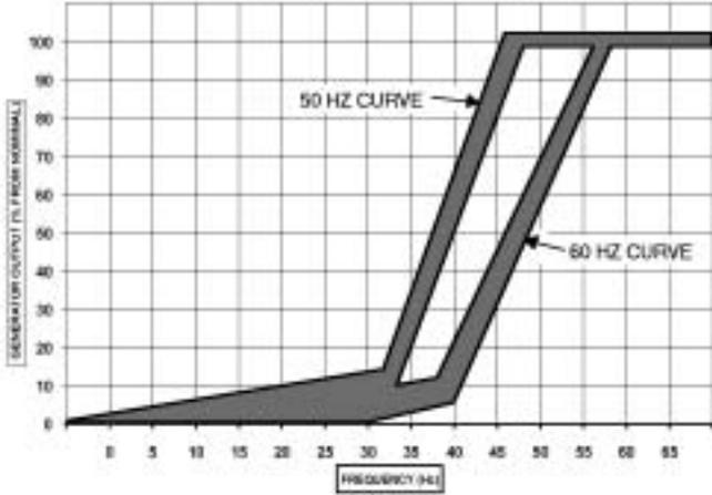
Figure 1. Frequency Compensation Curves
